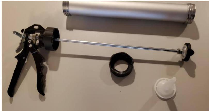
Figure 4: caulking gun disassembled
